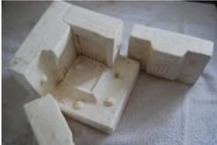
The mould taken from the original slab pot.
